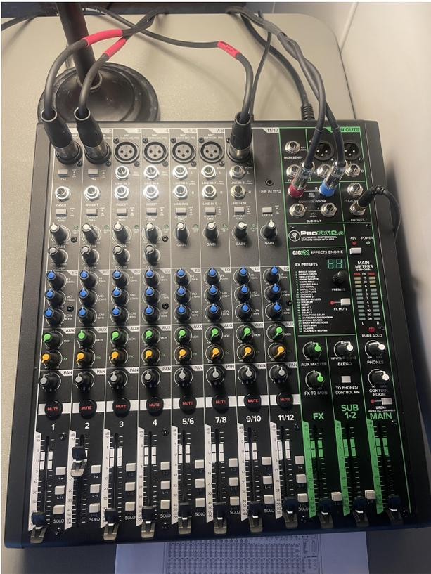
1. The 1/4" jacks plug into the *L/R Control Room* inputs on the mixer. The single jack on the cable's other end runs into the outer wall pocket. Another 1/4" cable runs from the inner wall pocket and into the *HA400 MicroAmp*.
