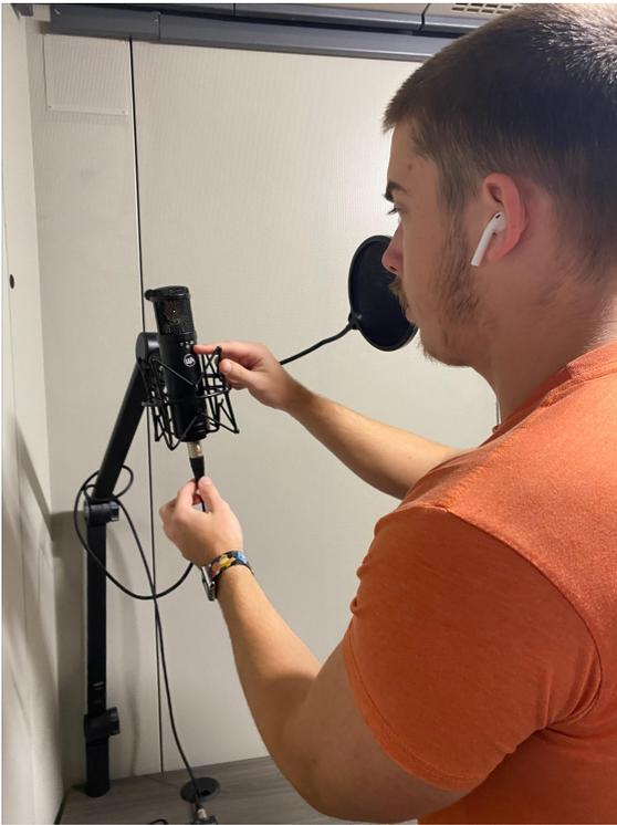
^The user is pointing at a switch on the WA-47 mic. This switch toggles between different polar patterns.^
