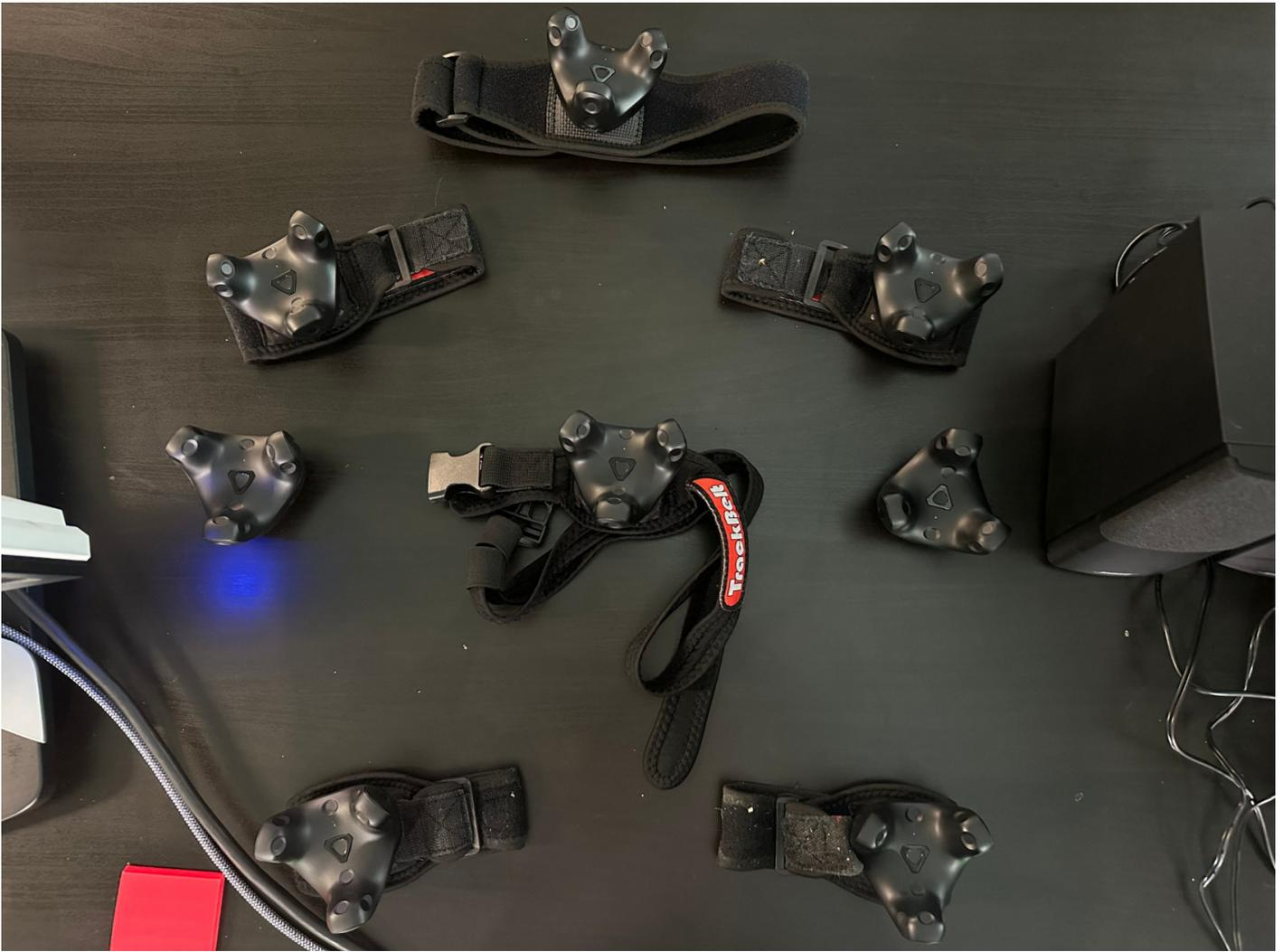
3. When affixing the trackers to the actor, ensure the LED light on each of the VIVE trackers that form a pair (such as the 2 upper arm trackers) aligns in the same direction as its corresponding device.
