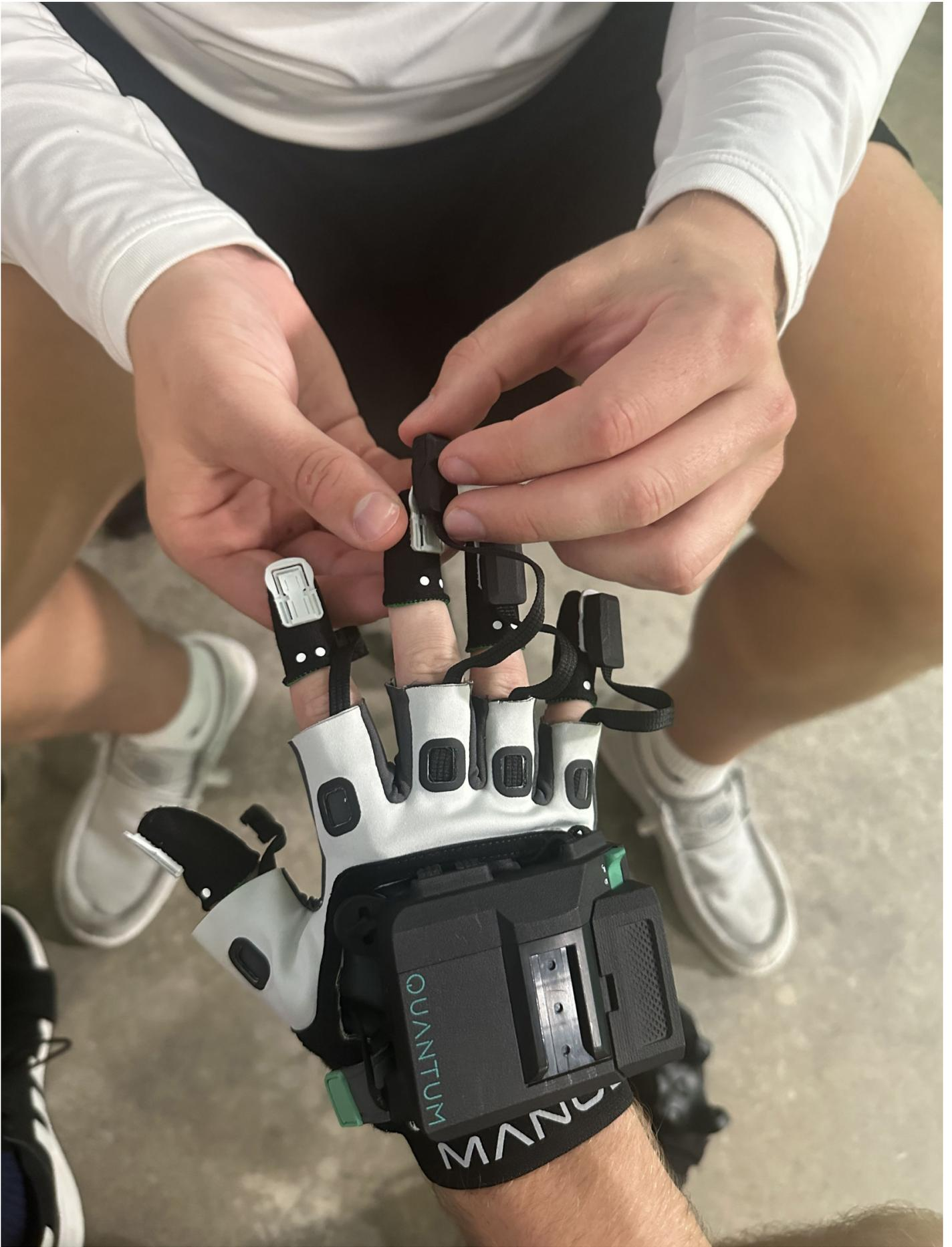
7. Locate the remaining two VIVE hand trackers and slide them onto the top of the gloves where the guard rail is located, one at a time. Slide each tracker until it locks into place or can't slide any further.
