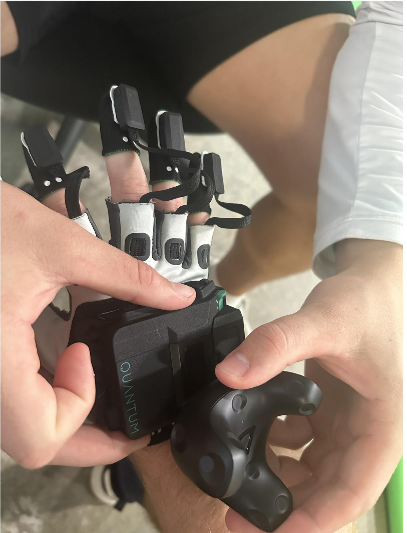
8. Thoroughly inspect both gloves and confirm with the actor that everything feels comfortable and secure. This may include adjusting the green side straps on the gloves for a tighter fit if necessary.
