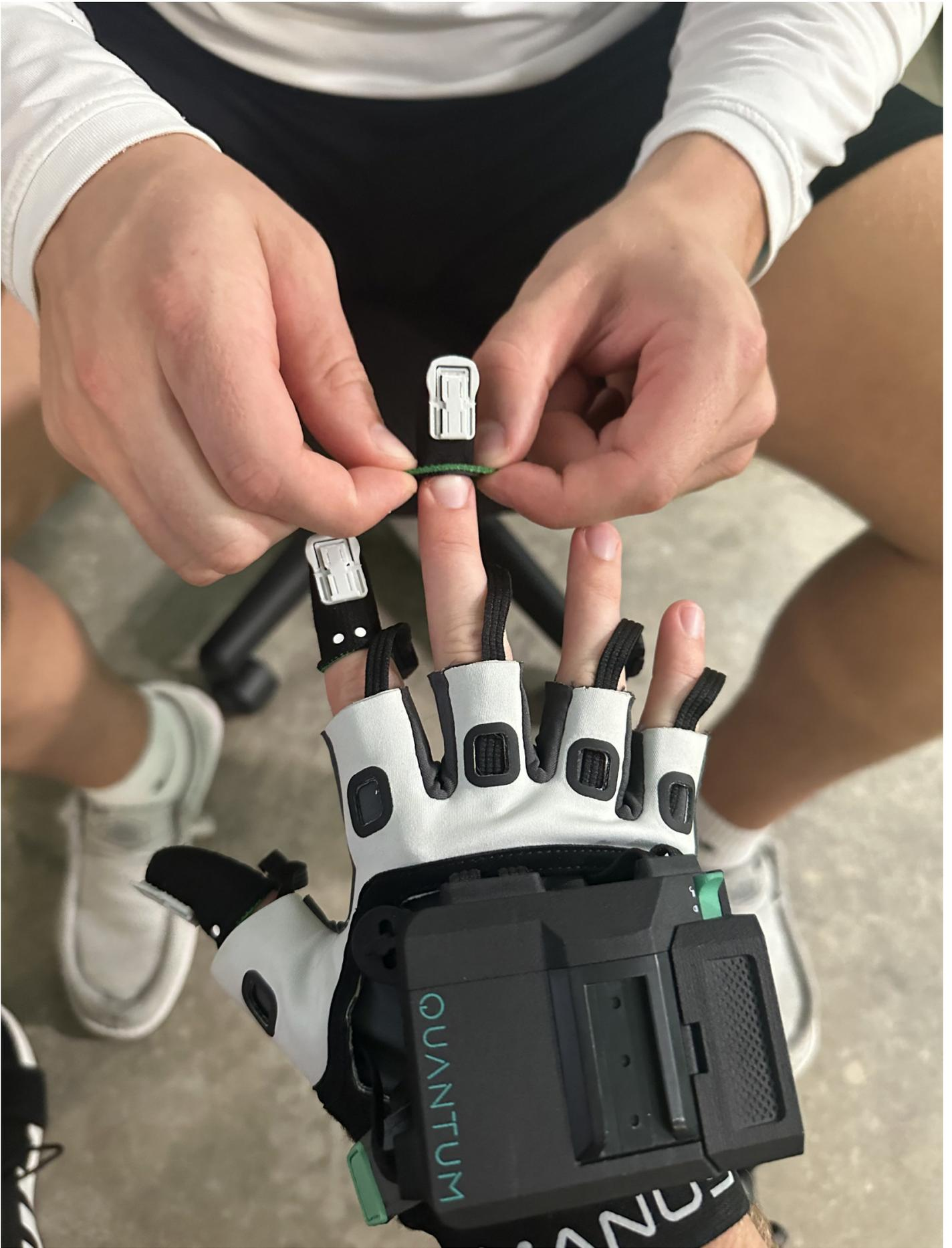
6. Attach the black sensor to each finger by sliding it onto the grey plastic slide rails attached to the fingertip covers. Do not allow the actor to perform this task; it requires two people to ensure proper and safe fitting. Slide the sensor until it locks into place or cannot slide any further.
