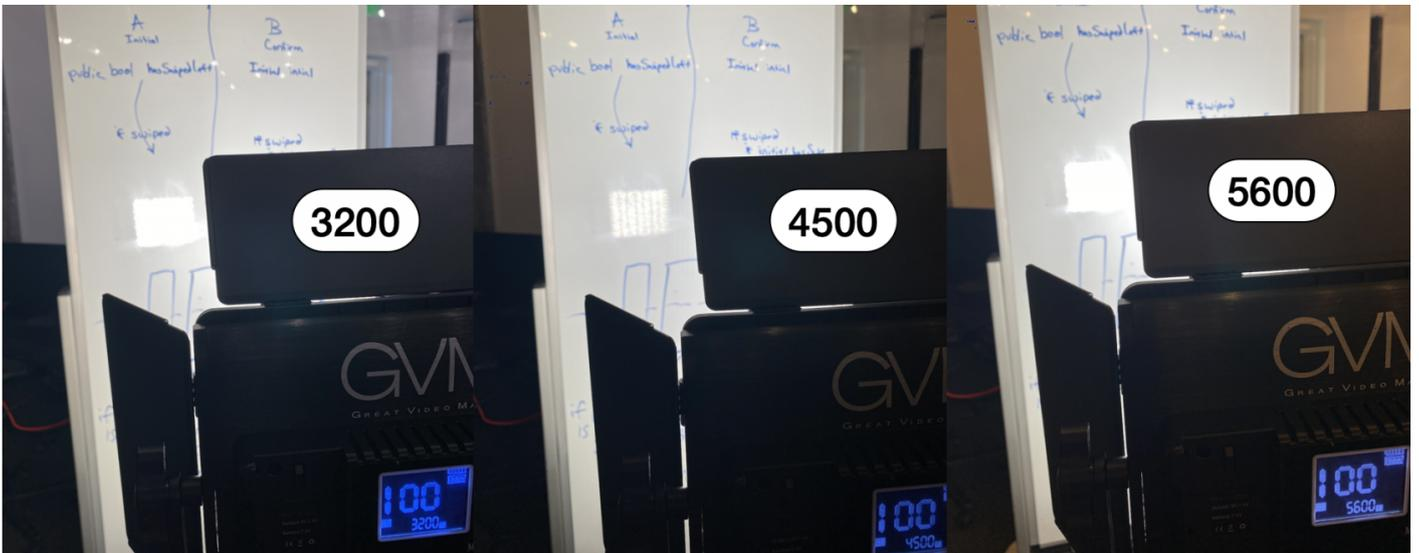
Hue: Use the right dial to adjust. The screen should display 'HUE' to adjust the color of the light. If not, press the right dial until it displays 'HUE'.
